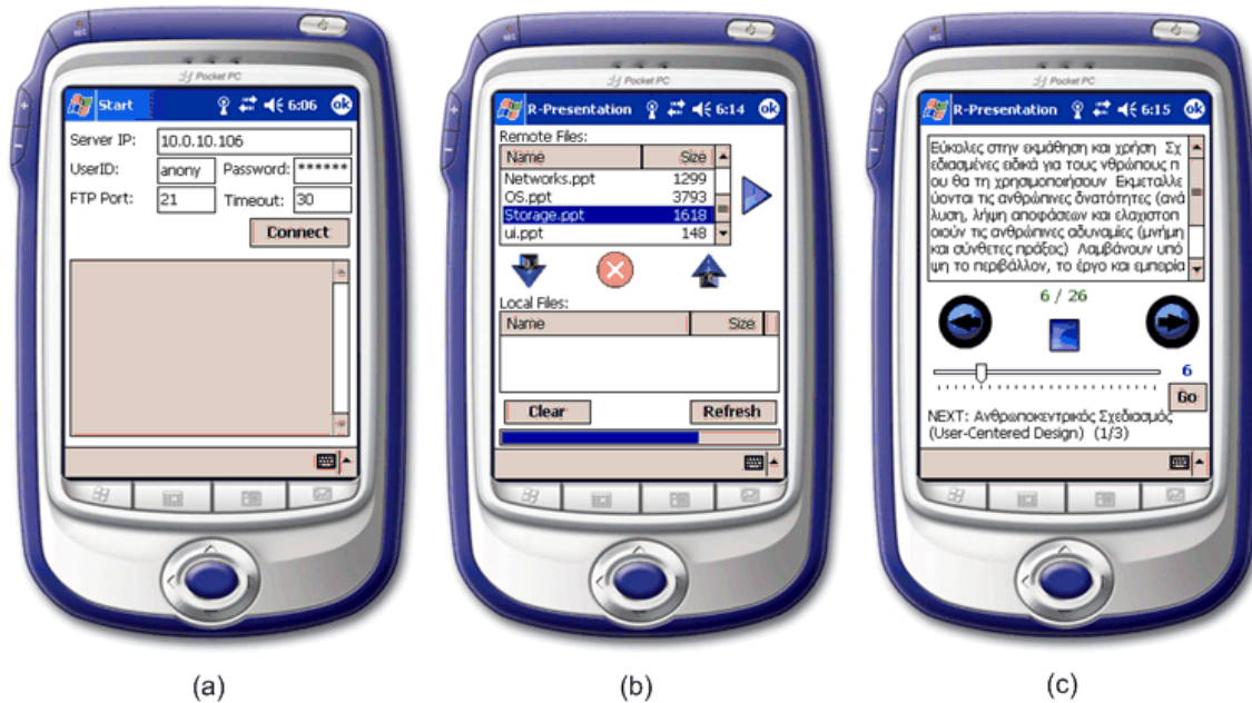
Figure 2: The User Interface of R-Client on the PocketPC 2003 Emulator – (a) Connect to R-Server, (b) Exchange files and load a presentation, (c) Navigate loaded presentation
