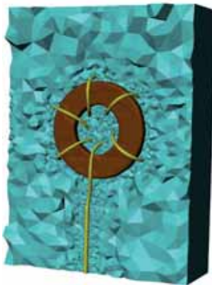
Fig. 2 - Generation of conforming multipart volume mesh of inductor core, wire and air in ScanIP+FE
