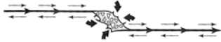
Figure 7.20 Arrows illustrate flow into a dilatational jog immediately following fault movement. (After Sibson, 1987, p. 702.)
