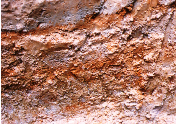
Figure 9 Yellowish orange with pale grey silty fine sand of second river terrace alluvium, Wong Kong Shan
