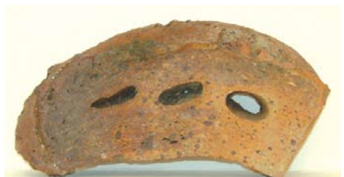
A distorted brick from Gloucester Brickworks. Poor quality clay caused expansion of gases during firing, leading to "blowing" of the bricks.
