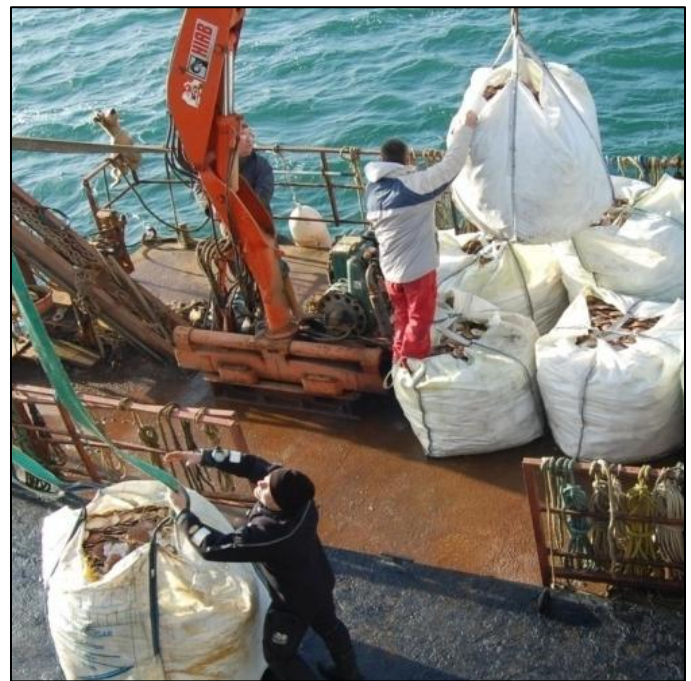
Fig 2. Cranes and barge used to lift and transport the 1 tonne scallop shell mesh bags.
