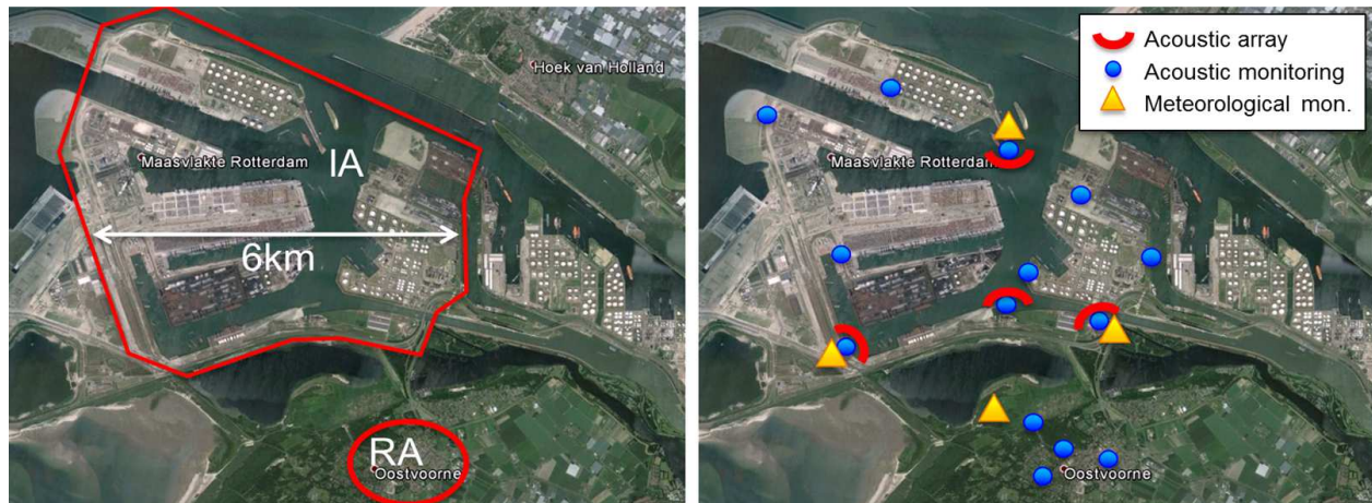
Figure 1: Maps showing (left) the Industrial Area (IA) and Residential Area (RA) and (right) the locations of multiple arrays and both acoustic and meteorological monitoring stations.
