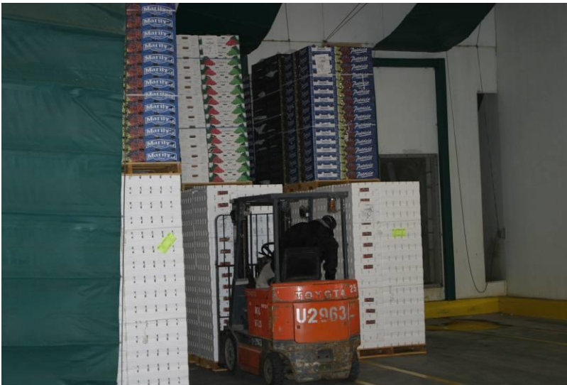
Photo 152. SO 2 gas room being filled with grape boxes.
