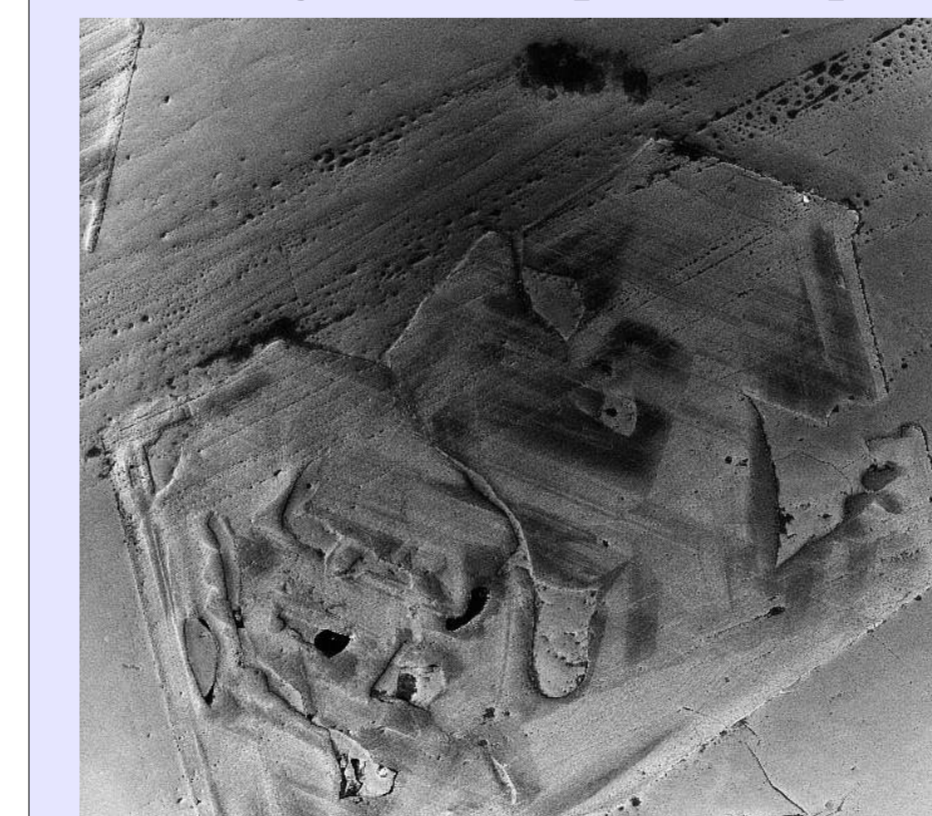
Fig. 18. Multiple sets of planar features in a moissanite crystal - possibly a shock effect. Field width 80 µm.
