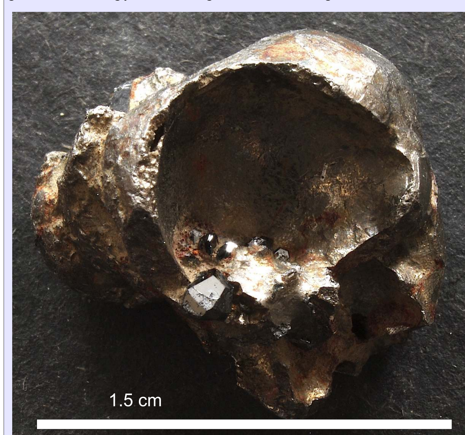
Fig. 2. The iron silicide matter from the Chiemgau region. A: small-sized metallic particles - angular and spherical. B: "Splash" form of iron silicide particles. C: SEM image of iron silicide perfect spherule. D: cubiform crystals paving the surface of an iron silicide particle. E, F: regmaglyptic surface of iron silicide particles. G: rear side of the particle in F. H: pyramidal shape of iron silicide particle.
