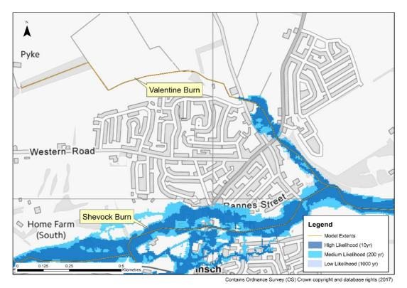
Figure 1-7: SEPA fluvial flood map extents for the Valentine Burn
