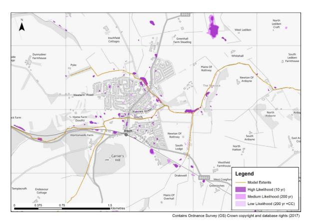
Figure 1-6: SEPA pluvial flood map extents for Insch
