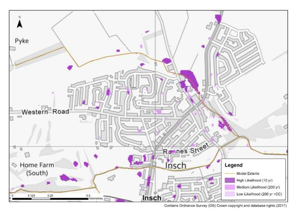
Figure 1-8: SEPA pluvial flood map extents for the Valentine Burn
