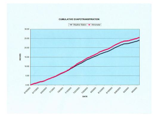
The field trial with OSU at Goodwell provided very similar results to the results in Graphs 1 and 2 above. The results in Graph 2 above indicated to NRCS that over a growing season, an atmometer can provide reasonable estimates of evapotranspiration similar to readings from a fully equipped weather station. Compared to a weather station costing thousands of dollars, the atmometer we found to be a simple and affordable device that could effectively be used by Oklahoma irrigators.
