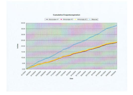
The results shown in Graph 3 indicated to NRCS that atmometers consistently provide accurate readings in comparison to each other when located at the same site. The results also indicated to us that an atmometer located in the same environment as an irrigators crop is a more valuable tool for scheduling than using readings from a remote weather station.
