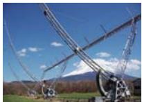
The radiotelescope at Fuji to observe the interplanetary scintillation.
