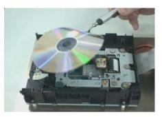
Fig.2 Thin film disk is put on the motor of commercialized standard BD drive.
