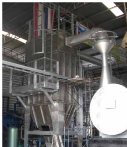
Therm Engineering, Tailandia Waste gas cleaning for garbage disposal plant separating of dust and sulphur dioxide
