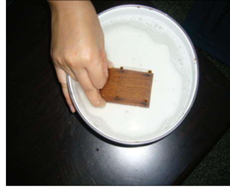
(a) Put the test boards into the liquid
