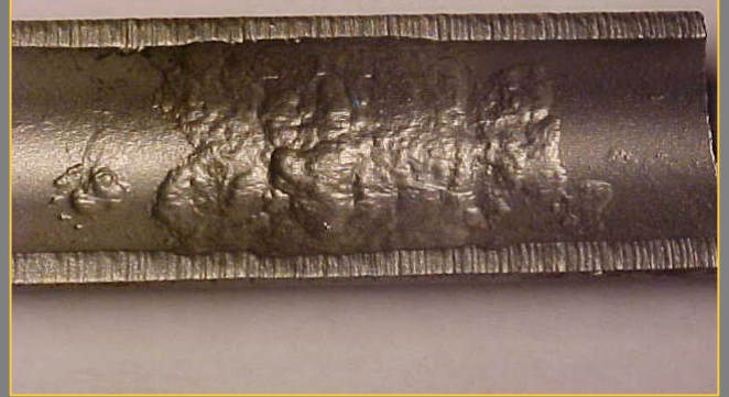
Tube sample (Aluminum fins removed) – heavy corrosion concentration
