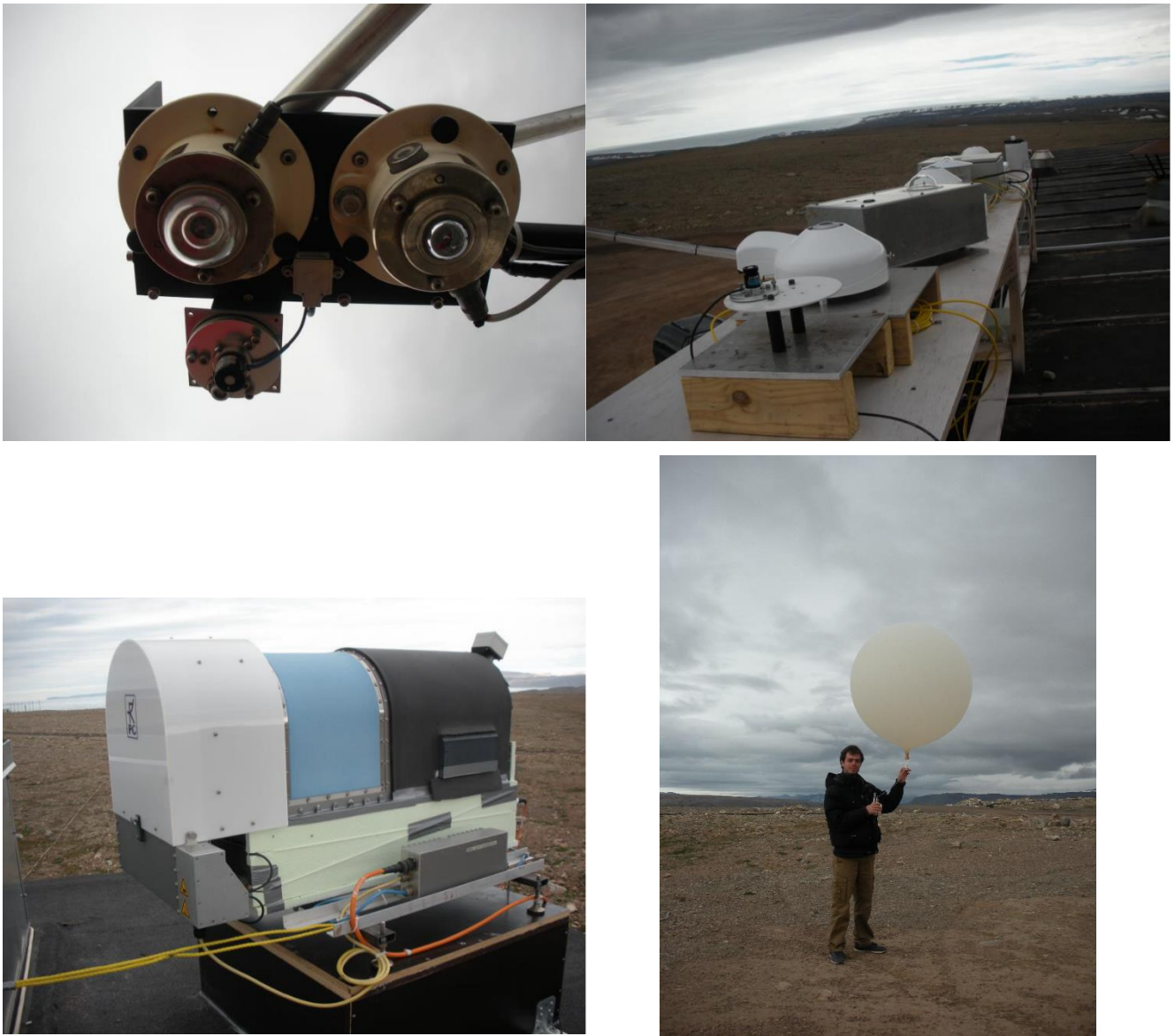
Figure 6.2: Top left and right: down-looking and up-looking radiometers, bottom left: the HATPRO radiometer, bottom right: a radiosonde launch.
