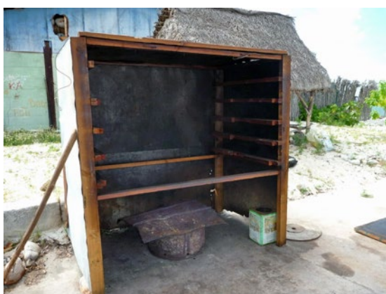
Figure 4. A smoke house on Tarawa, Kiribati, for smoking sea cucumbers. The sea cucumbers are placed on mesh trays that slide into the oven and sit well above a smouldering fire.
