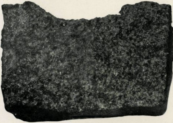
FIG. 2. Fractured surface of the same stone, showing its crystalline structure.
