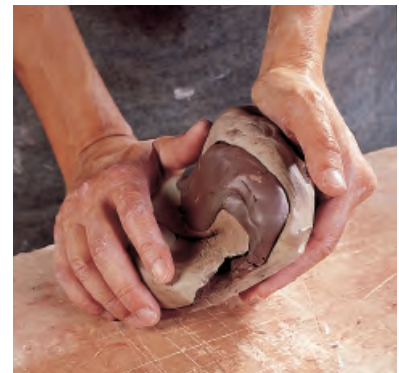
Figure 20 The clay is carefully wedged or kneaded to prepare it for throwing. Care has to be taken at this stage to expel air from the clay without overworking the clays. The more the clays are wedged the less distinct the resulting agate pattern.
