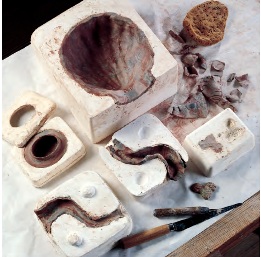
Figure 56 The two piece molds necessary for producing a pecten shell teapot including the body, spout, handle, and Fo Lion finial. These molds were taken from original master models sculpted by Michelle Erickson.
