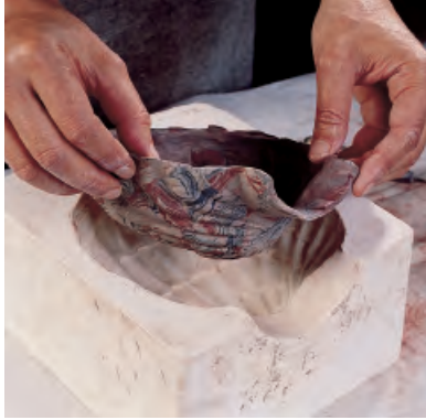
Figure 55 The slab is allowed time to firm up within the mold so the completed teapot half being removed is without distortion.
