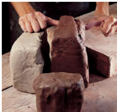
Figure 18 In preparing the clay for throwing an agateware mug, slabs of varied colored earthenware clays are cut and stacked. At this stage the proportion of the colored clays determine the intensity of the agate patterning. Three colored clays are selected for making a mug: a white clay, a red iron clay, and an iron manganese body.
