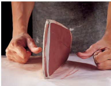
Figure 34 The combined clay slab is cut in half and the two pieces restacked. This process is repeated, continuously adding and thinning the layers.
