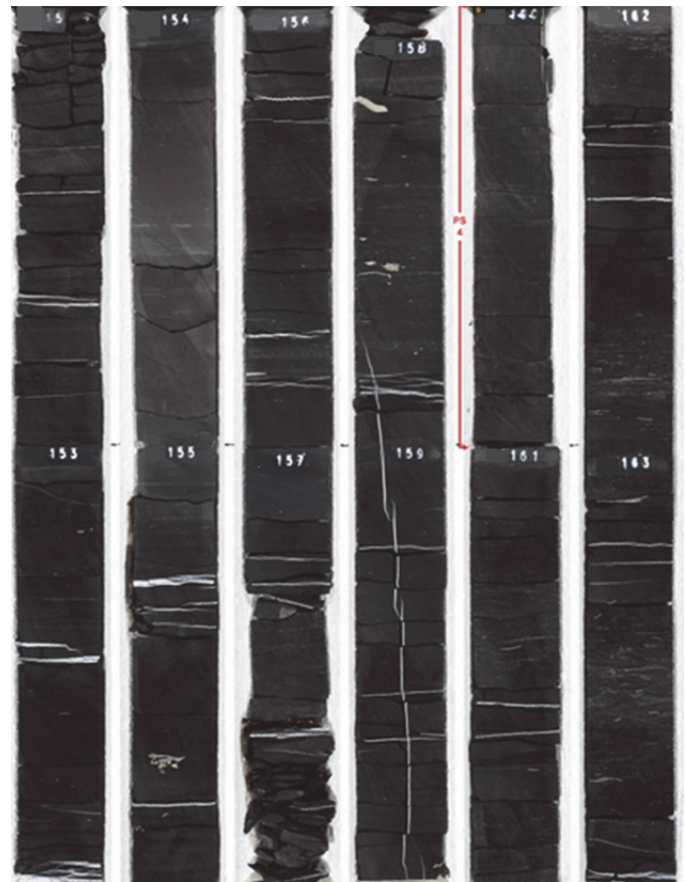
Fig. 4. Photograph of vertical core taken through the reservoir showing a sub-vertical calcite-filled natural fracture. The frequency of these fractures in the core is approximately every 6 meters (20 feet) indicating a relatively high fracture intensity in the reservoir, but they were invisible to the crossed-dipole sonic logging tool.
