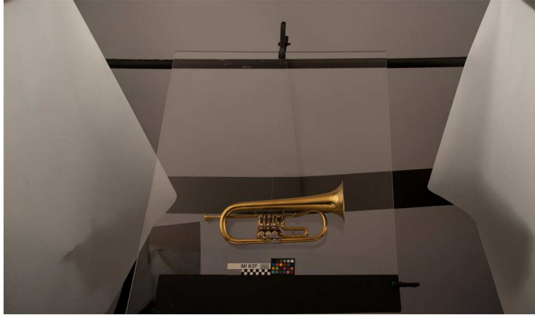
Plexiglas background device, here for trumpets. The black stripe in the background retaining unwished reflections doesn't appear in the final visual field. The instrument is secured from slipping away on the inclined surface by a nylon wire fixed on the black clamp on top of the Plexiglas sheet. photo GNM
