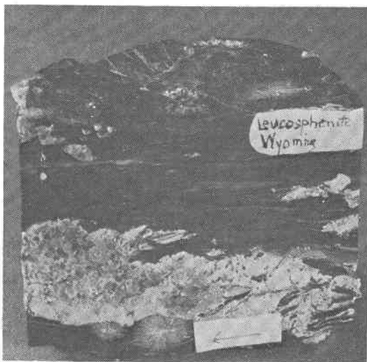
FIG. 5. Section of 2½-inch drill core from the Green River Formation, Wyoming, showing vein of shortite and loughlinite and two rosettes of leucosphenite enclosed in oil shale. Larger rosette (near arrow) is 1 cm in diameter.
