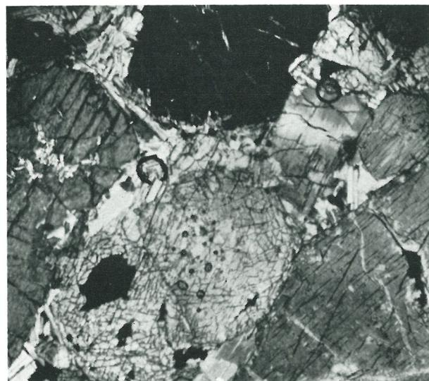
FIG. 5. Close packed hypersthene with interstitial bytownite, Mt. Harmsworth Dike, (16790)  $\times 30$ .
