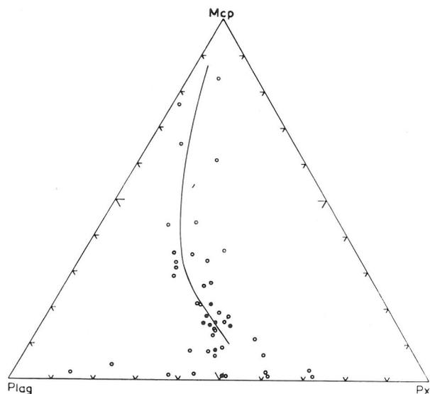
FIG. 1. Triangular diagram of modal plagioclase, pyroxene and micropegmatite plus remaining phases in 46 specimens of Ferrar Dolerite. Solid circles represent undifferentiated rocks. Plagioclase and hypersthene cumulates are at the base and granophyres and pegmatoids near the upper apex.
