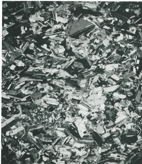
FIG. 4. Photomicrograph, of anorthosite, Mt. Egerton Sill (16797). A little augite is ophitically intergrown with the bytownite which shows a roughly parallel orientation.  $\times 30$ .
