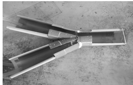
FIG. 1. Y-maze used in the chemical orientation experiment. Both arms of the Y-maze were 30 cm long, and the base was 26 cm long. The Y-maze was 5 cm wide and 4 cm deep.
