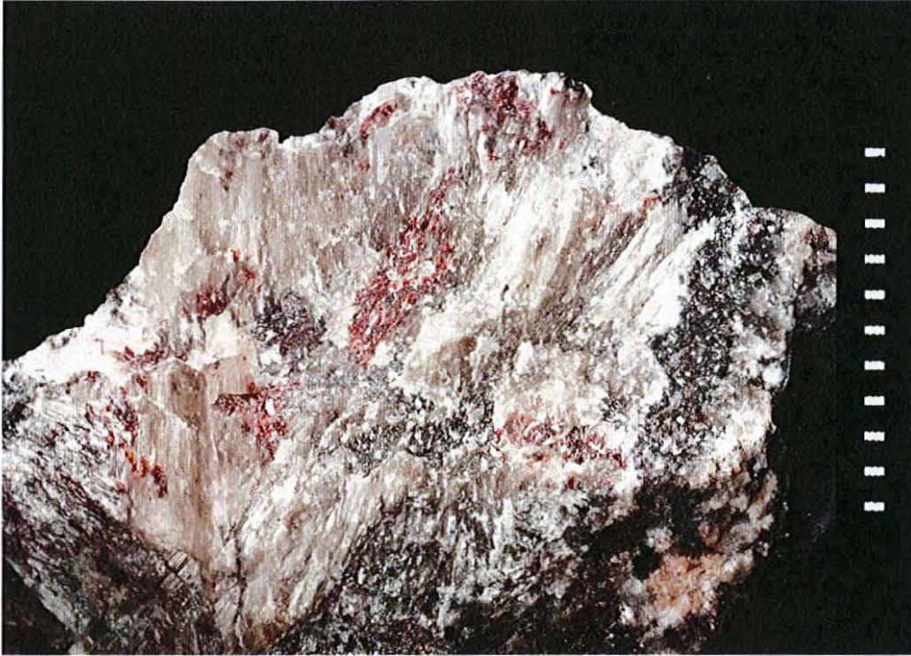
Fig. 7. Red parkinsonite within striated mendipite, with minor black plattnerite from the collections at the NHM. Scale bar divisions are equal to 1 mm.
