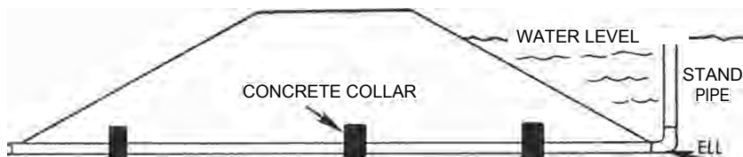
Figure 2. Cross section of a dam showing the drain pipe with concrete collars to prevent seepage, and a threaded standpipe for draining the pond.
