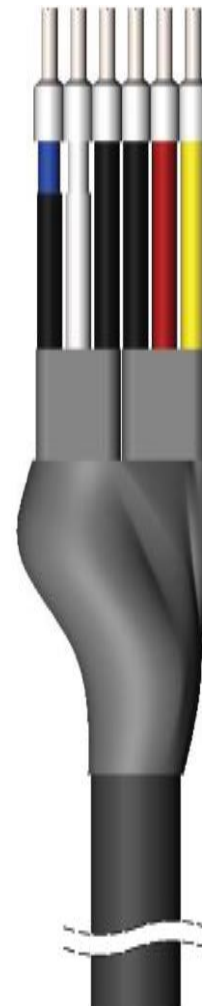
Figure 19: SPI Cable Wires
