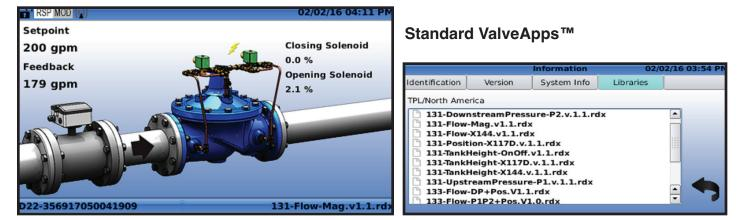
At startup the user can select from an internal library of Standard ValveApps designed for the most common control applications such as flow, pressure, level, position, or pressure management. Pre-configured graphics displays actual valve installation and minimizes startup time.
