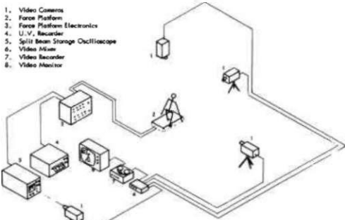
Fig. 5. Schematic diagram of gait analysis apparatus.
