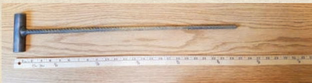
A live stake pilot hole driver pictured alongside a measuring stick to scale. A live stake pilot hole driver (a piece of scrap rebar with a welded handle to help push the rebar in and pull it out). Photo by Ryan Davis
