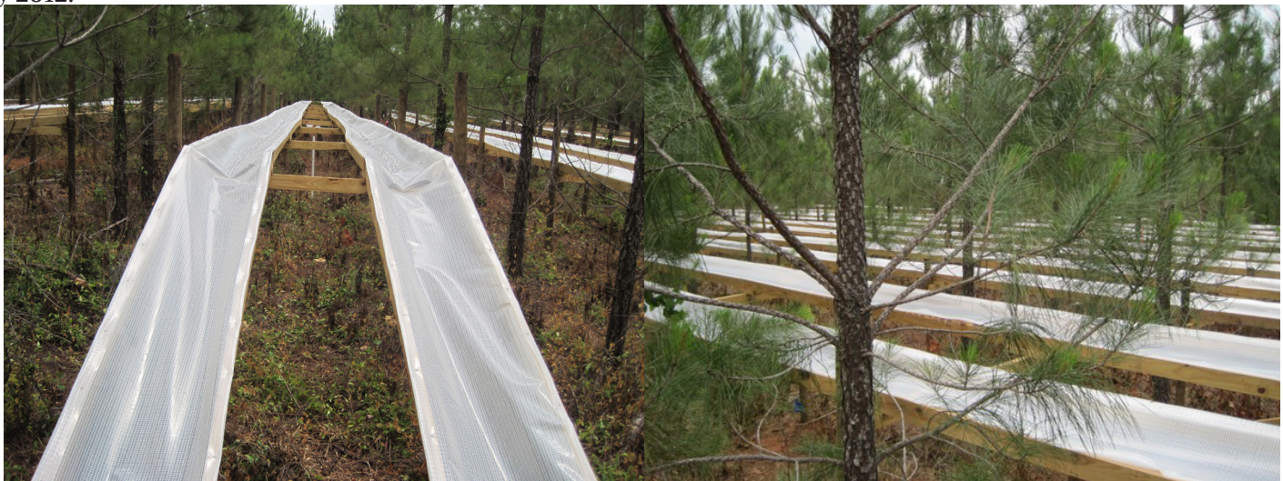
Figure 2. Throughfall exclusion structures at the Tier III site in Tallapoosa County, Georgia. Photos by Madison Akers.
