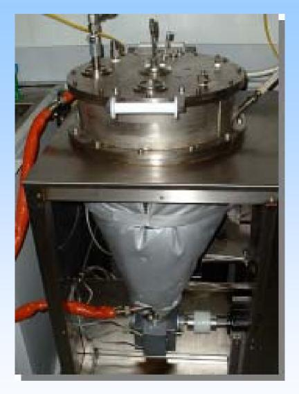
Electrically Heated Reactor 30cm disc diameter with conical walls Variable speed of up to 1200rpm
