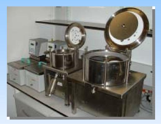
Fluid Heated / Cooled Reactors 10cm and 20cm disc diameter Variable speed of up to 3000rpm
