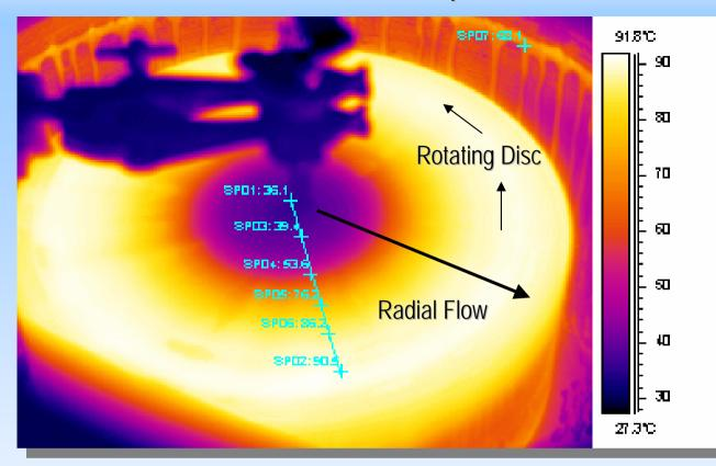
Continuous heating of "Treacle" from 40°C to 90°C in seconds using a SDR
