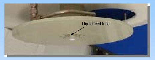
Polypropylene shroud plate to direct gas flow over the rotating disc.
