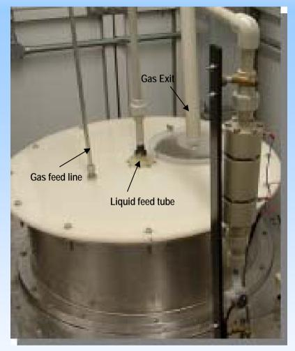
30cm SDR with built-in conductivity monitor for measuring ion depletion during conversion
