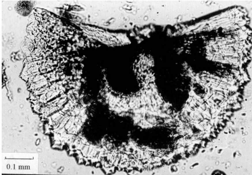
Fig. 9. Fragment of a spherulitic aggregate of acicular crystals of harmotome intergrown with smectite (black parts). Red beds of the "Marcel" mine. Grain mount; polarizing microscope; one polar
