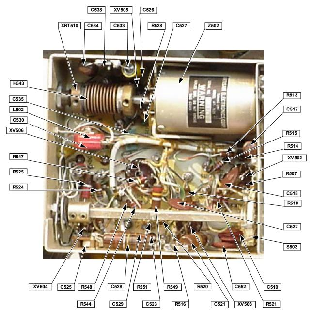
Figure 6-17 IF Subchassis, Front Section 13
