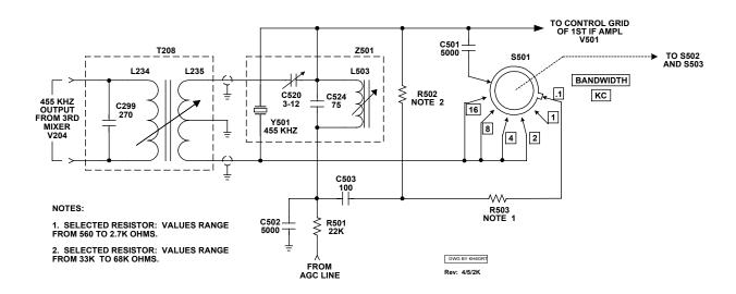
Figure 3-4 Crystal Filter, Simplified Schematic Diagram<sup>4</sup>
