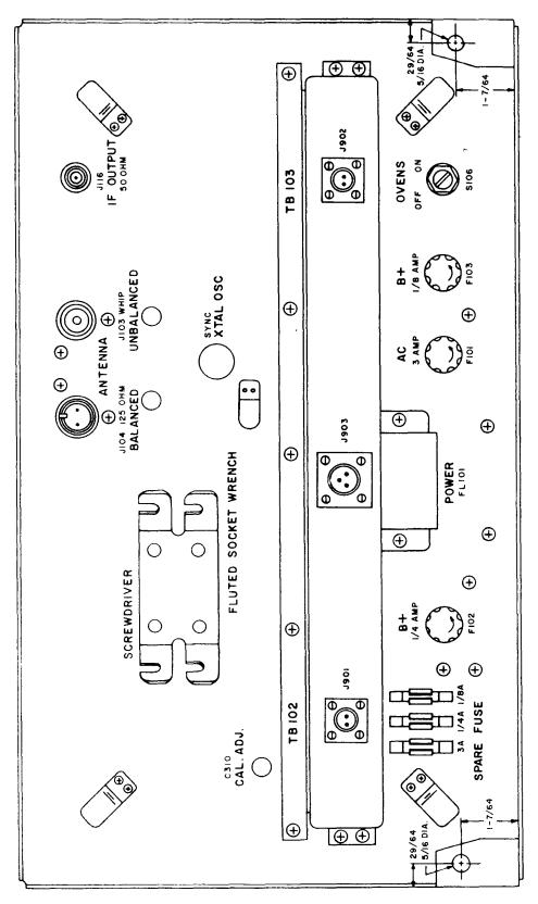
Figure 2-3 - Rear Panel for Shipboard Use
