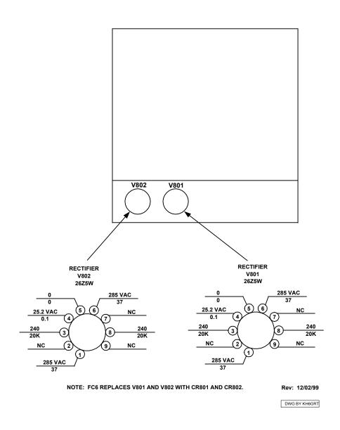
Figure 5-9 Power Supply Sub-chassis, Voltage and Resistance Diagram<sup>9</sup>
