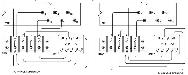
Figure 8-3 - Connections for 115-Volt or 230-Volt Operation<sup>1</sup>
