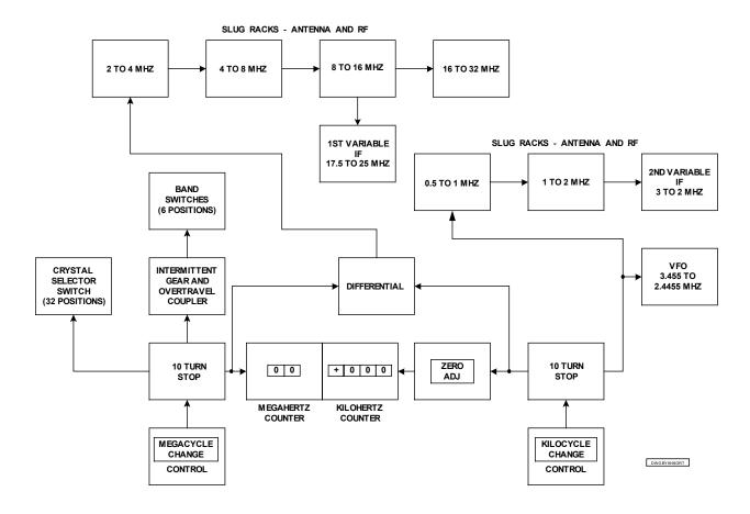
Figure 3-9 Tuning System, Mechanical Block Diagram<sup>7</sup>
