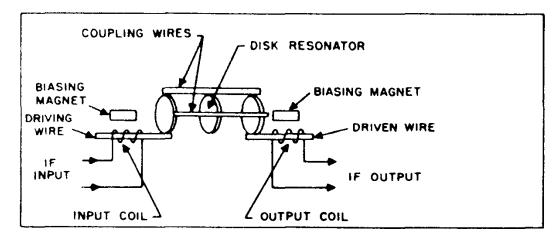
A. COMPONENTS OF A MECHANICAL FILTER
