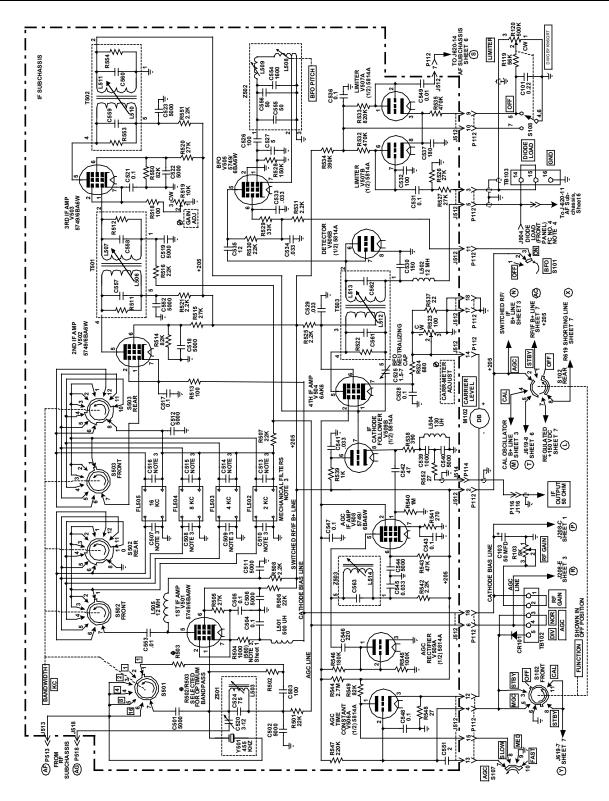
Figure 5-22 Schematic Diagram, Part 5 of 7 - IF Amplifiers, AGC, Limiter and Detector<sup>23</sup>
