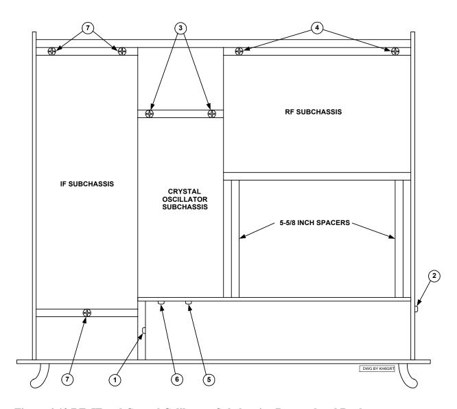
Figure 6-10 RF, IF and Crystal Calibrator Subchassis - Removal and Replacement, Location of Screws  $^8$
