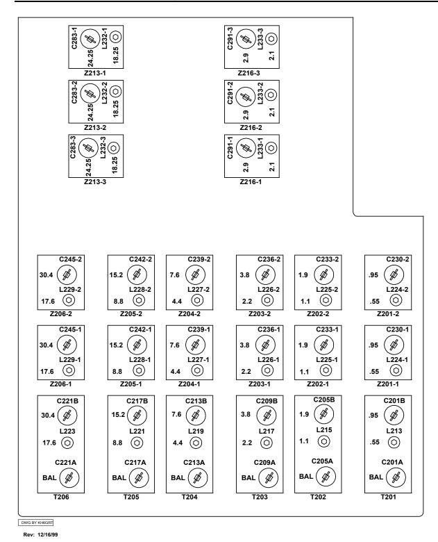
Figure 6-6 RF and Variable IF Alignment Points<sup>4</sup>
