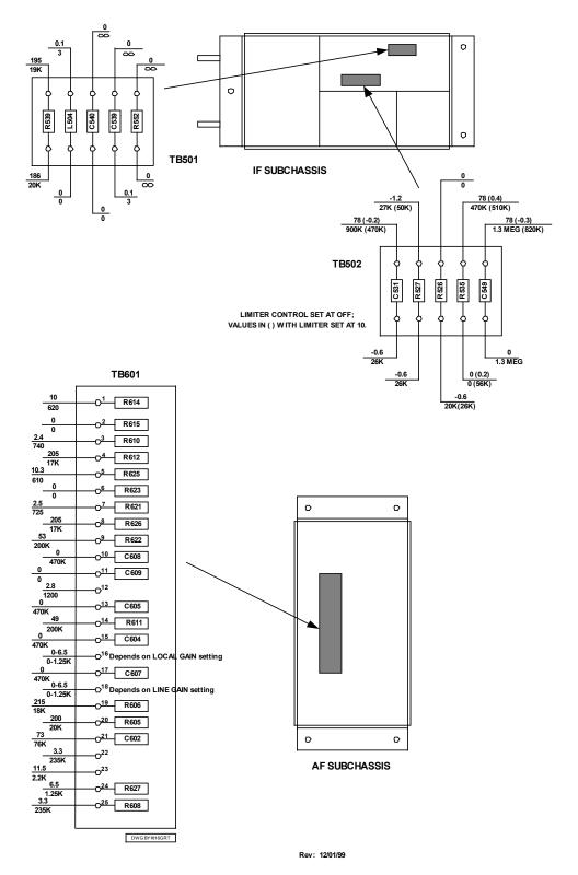
Figure 5-10 IF and AF Sub-chassis Resistor and Capacitor Terminal Boards, Voltage and Resistance Diagram<sup>10</sup>
