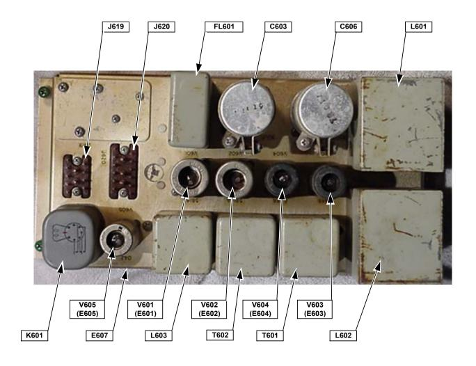
Figure 6-27 AF Subchassis, Top View<sup>18</sup>
