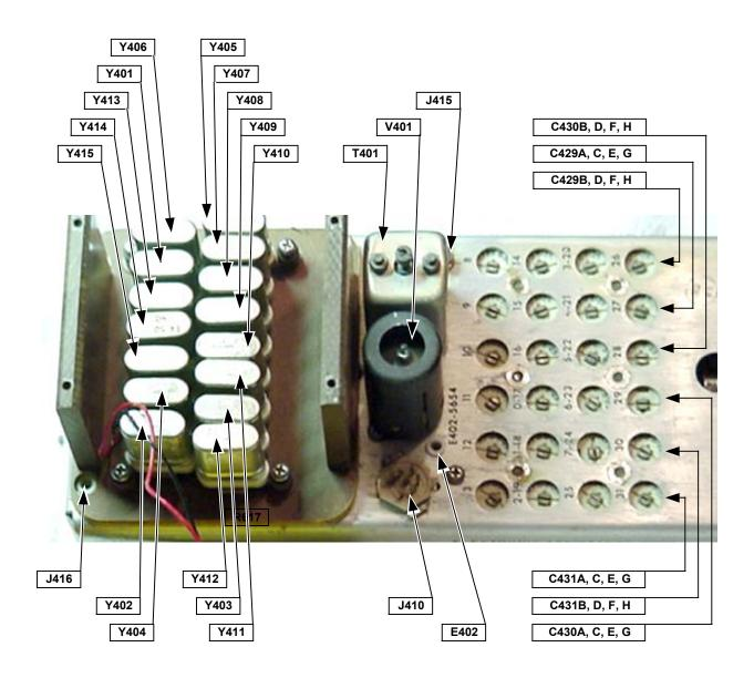
Figure 6-22 Crystal Oscillator Subchassis - Top View<sup>15</sup>
