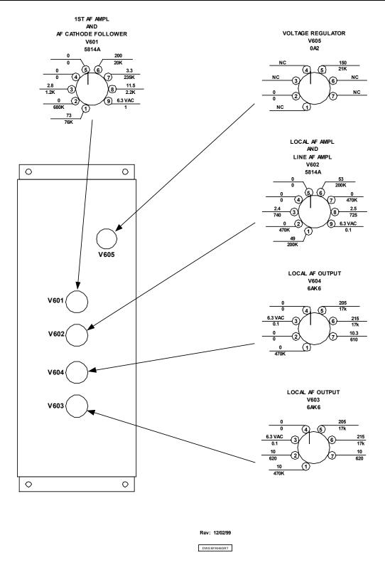
Figure 5-8 AF Sub-chassis, Voltage and Resistance Diagram<sup>8</sup>
