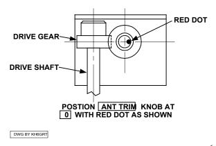
Figure 6-8 ANT TRIM Control Adjustment<sup>6</sup>
