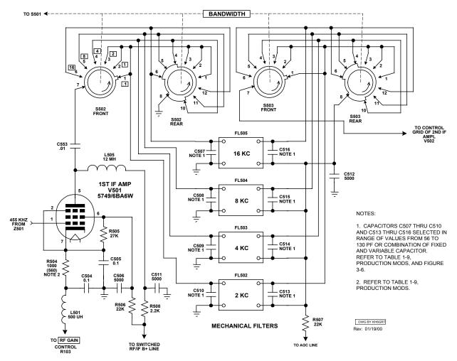
Figure 3-5 First IF Amplifier V501, Simplified Schematic Diagram<sup>5</sup>
