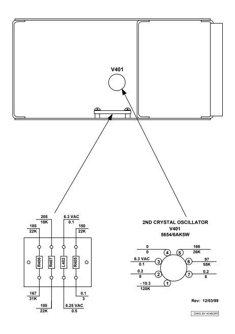
Figure 5-5 Crystal Oscillator Sub-chassis, Voltage Resistance Diagram<sup>5</sup>
