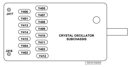
Figure 6-12 Location of Crystals Y401 through Y415<sup>10</sup>
