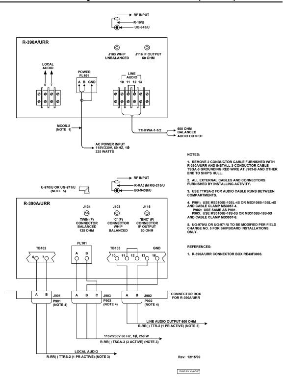
Figure 8-4 - Interconnecting Cabling<sup>2</sup>
