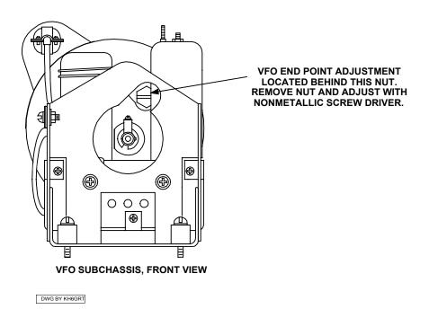
Figure 6-7 Variable Frequency Oscillator End-Point Adjustment<sup>5</sup>
