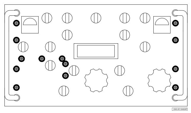
Figure 6-9 Location of Front Panel Mounting Screws<sup>7</sup>
