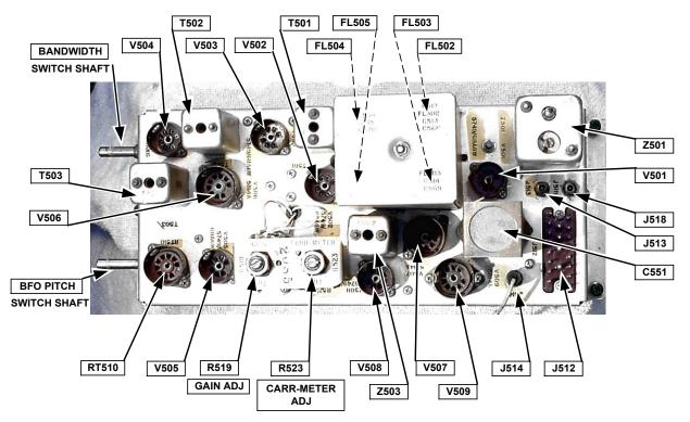
Figure 6-16 IF Subchassis, Top View<sup>12</sup>
