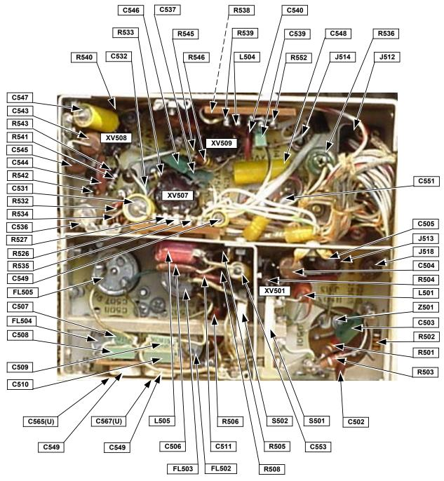
Figure 6-18 IF Subchassis, Rear Section<sup>14</sup>
