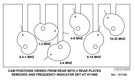
Figure 6-13 RF Gear Train Assembly Cam Positions Viewed From rear, Simplified Mechanical Diagram<sup>11</sup>
