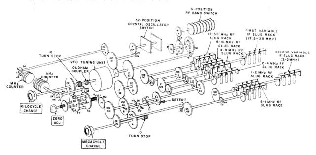
Figure 3-10 Tuning System, Simplified Mechanical Diagram
