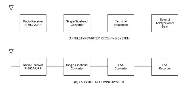
Figure 1-2. System Applications for Teletypewriter and Facsimile Equipment<sup>1</sup>
