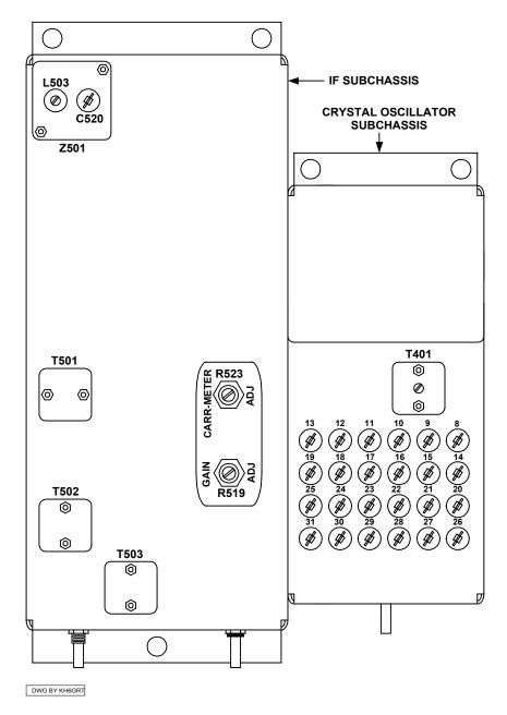
Figure 6-5 Crystal-Oscillator and IF Subchassis Alignment Points<sup>3</sup>
