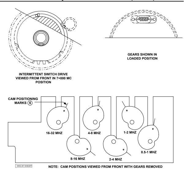
Figure 6-2 Mechanical Alignment Details<sup>1</sup>
