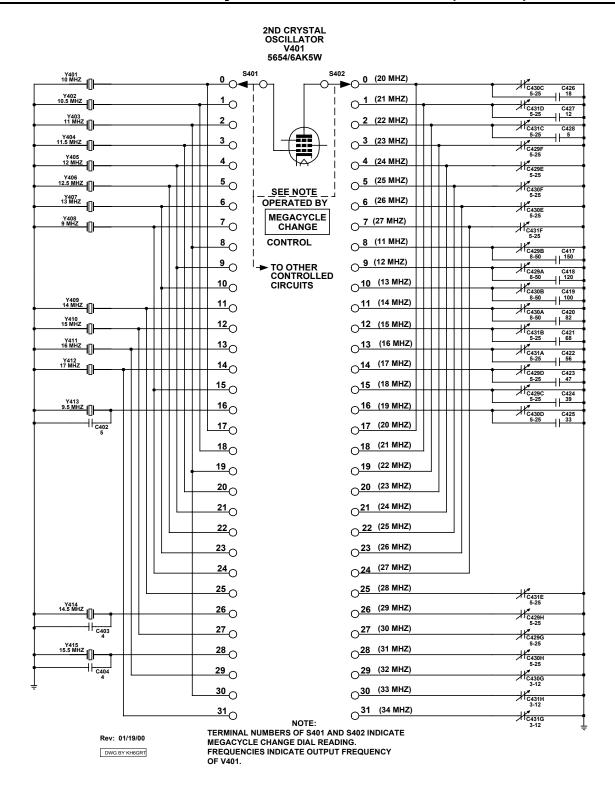
Figure 3-3 Second Crystal Oscillator V401, Crystal and Plate Circuit Switching Schematic Diagram<sup>3</sup>
