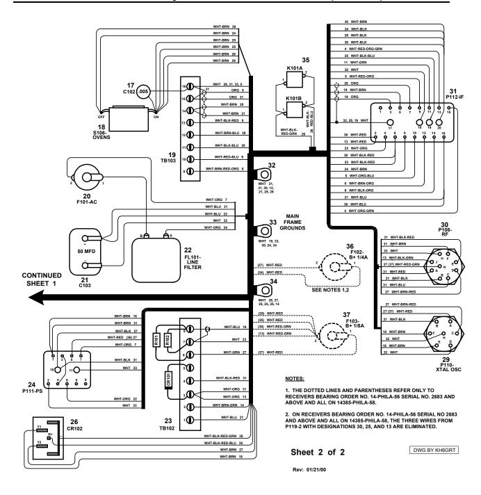
Figure 6-35 Radio Receiver R-390A/URR, Main Frame Wiring Diagram (Sheet 2 of 2)<sup>25</sup>
