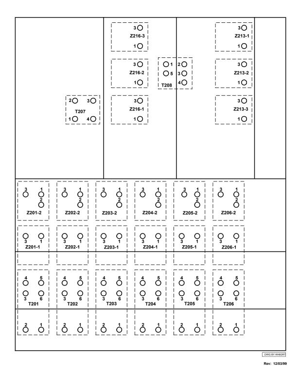
Figure 5-1 Terminal Numbers of RF and Variable IF Coils<sup>1</sup>
