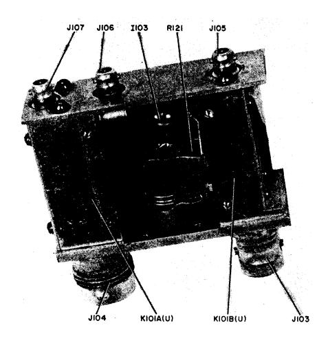
Figure 6-31. Antenna Relay Assembly, Internal View
