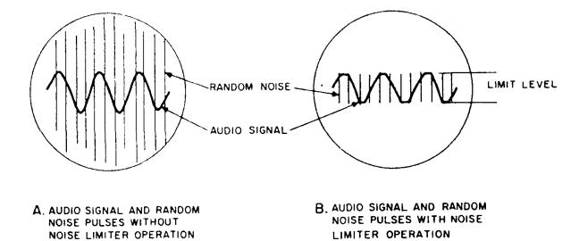
Figure 3-8 Typical Oscilloscope Presentations of Limiter Operation
