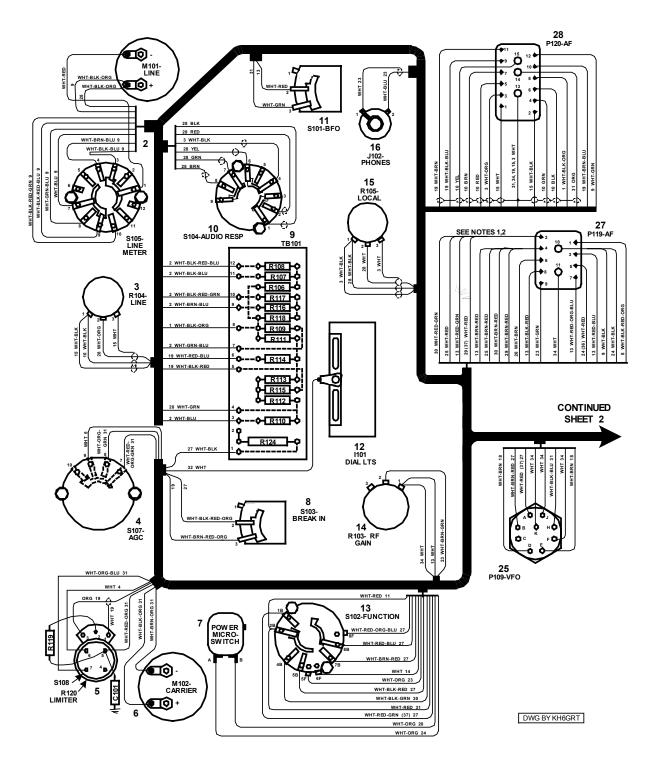
Figure 6-35 Radio Receiver R-390A/URR, Main Frame Wiring Diagram (Sheet 1 of 2)<sup>24</sup>
