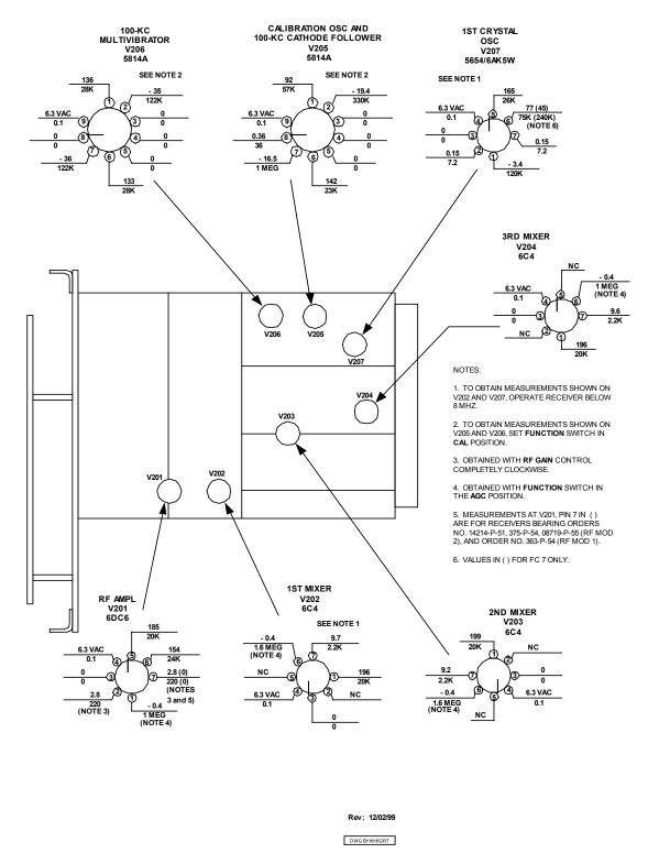
Figure 5-4 RF Sub-chassis, Voltage and Resistance Diagram<sup>4</sup>
