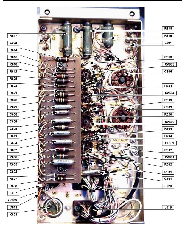
Figure 6-28 AF Subchassis, Bottom View<sup>19</sup>
