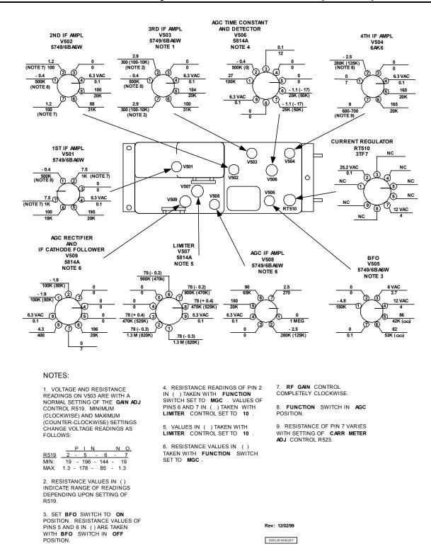
Figure 5-6 IF Sub-chassis, Voltage and Resistance Diagram<sup>6</sup>
