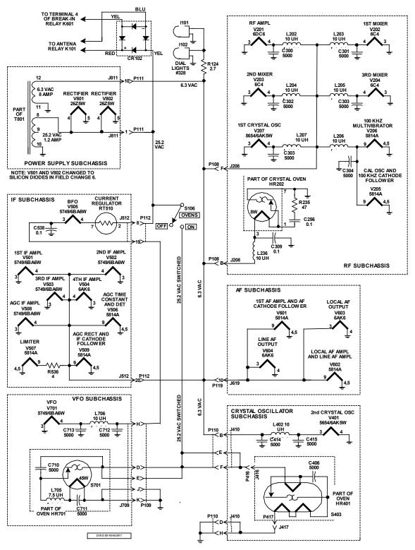
Figure 5-12 Filament and Oven Circuits<sup>12</sup>
