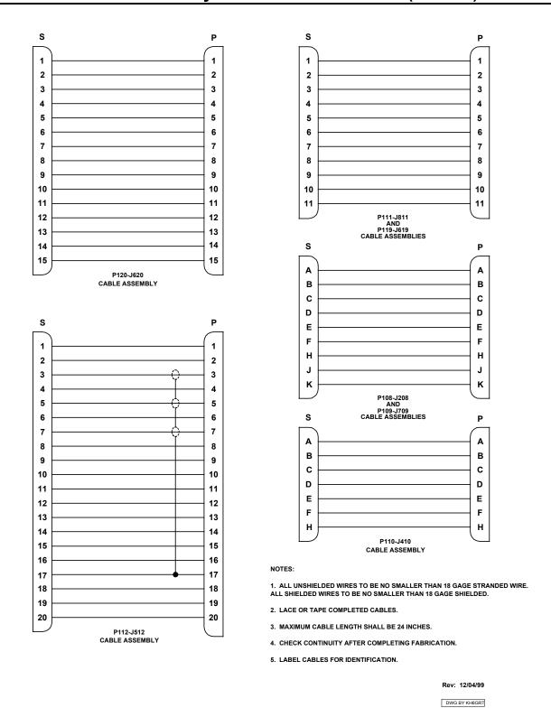
Figure 5-3 Fabrication of Multi-conductor Test Cables<sup>3</sup>
