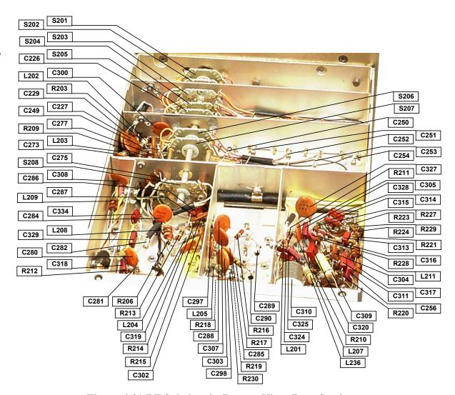
Figure 6-21 RF Subchassis, Bottom View, Rear Section
