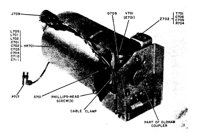
Figure 6-25. VFO Subchassis, Top View
