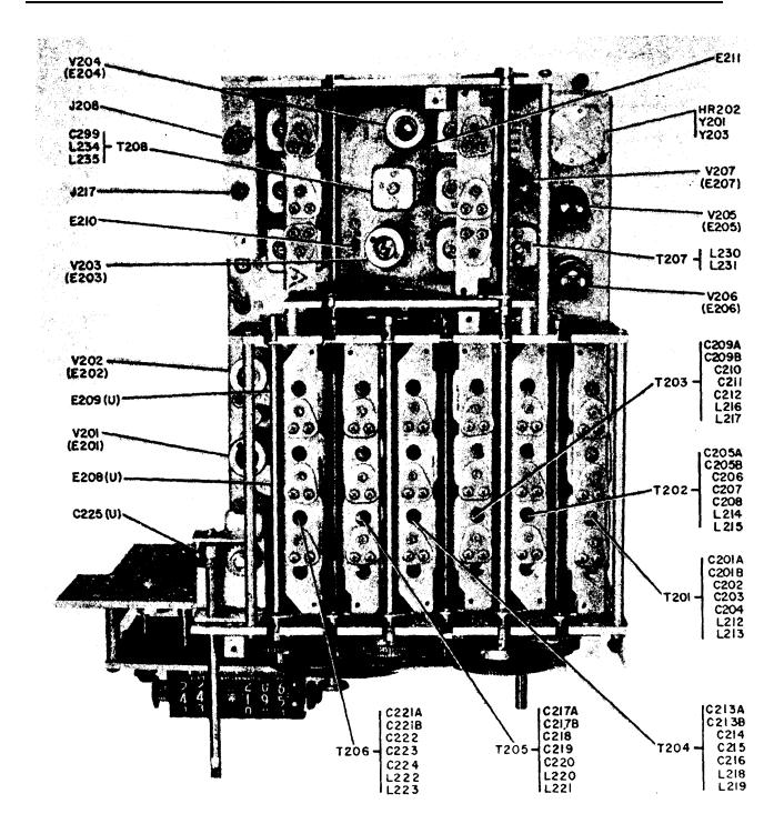
Figure 6-19. RF Subchassis, Top View (Sheet 1 of 2)
