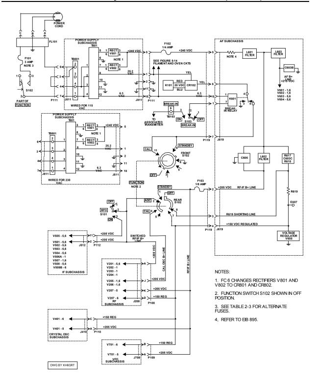
Figure 5-11 Power Distribution Diagram<sup>11</sup>
