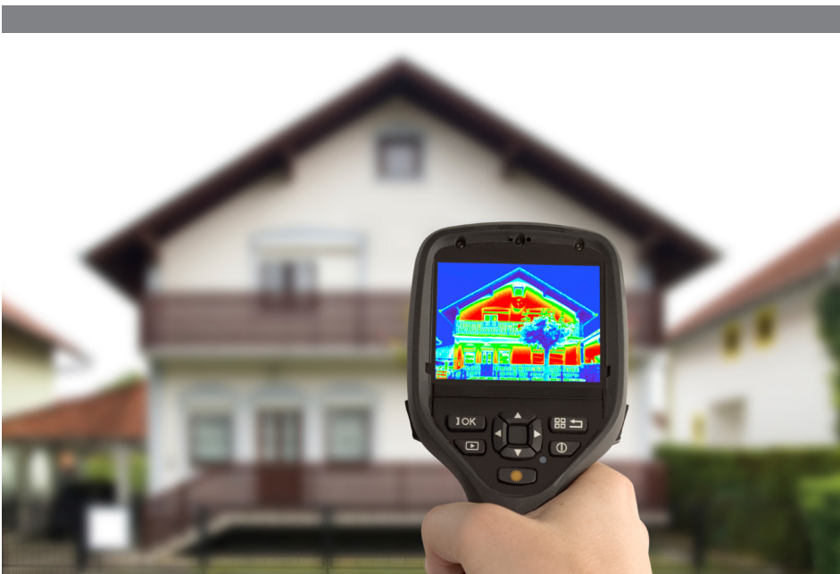
Thermal imaging camera used to detect heat loss in homes and to determine solutions for building efficiency.
