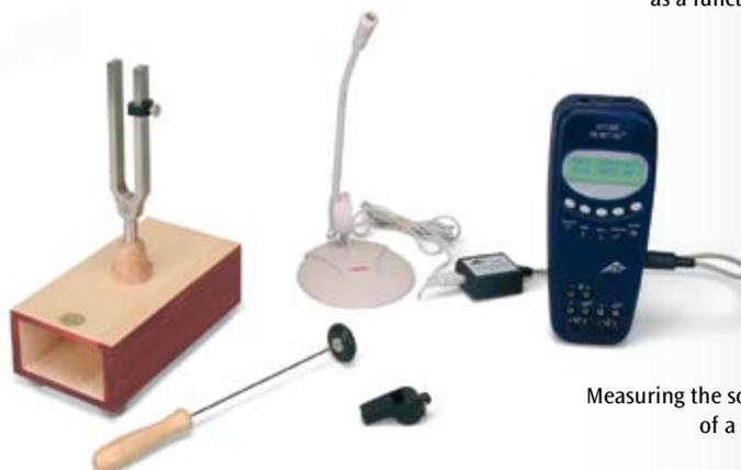
Measuring the sound waves of a tuning fork
