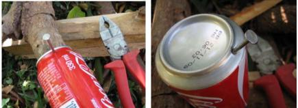
The can is placed over a log or pole which makes the hole easy to make with a nail. Two holes are made on either side of the can at the top. Then a single hole is punched into the base of the can in a position between the two holes at the top of the can. A good nail diameter is 3mm.
