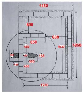
Dimensions of the brick square spiral BVIP in mm.
