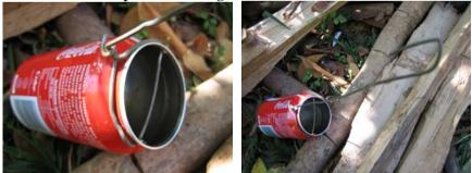
A length of wire about 30cm long is then taken and passed through the two holes at the top of the can. The wires are twisted together behind the can as shown. A loop is made at the end of the wire. The hand washer is hung from another wire attached to the toilet roof.
