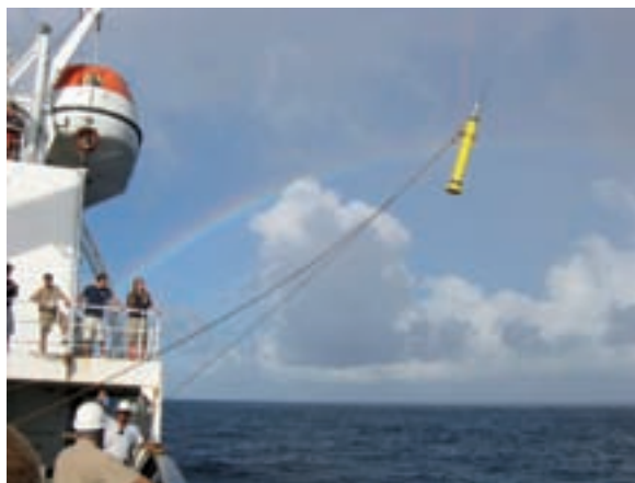
Figure 24. Deployment of an Argo float. The international Argo project has established a global network of more than 3,000 profiling floats. (©Euro-Argo)
