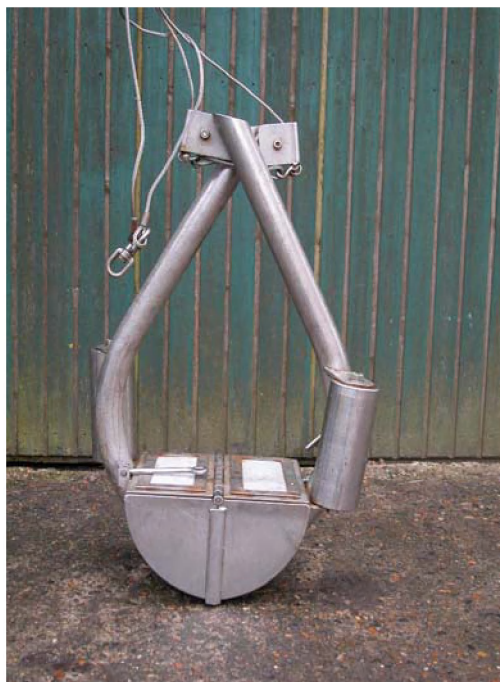
Figure 3. Van Veen grab of the Senckenberg Institute, Germany
