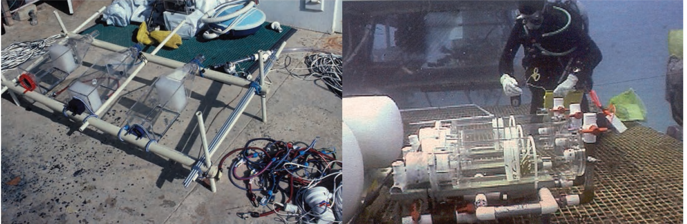
FIGURE 6. Respirometry chambers used for coral production and respiration measurements at a range of flow speeds being prepared for use in Hydrolab by M. Patterson and colleagues (left) (Patterson et al., 1991; photo by Kenneth Sebens), and similar chambers being used for nutrient uptake studies (right) (Leichter et al., 2003; photo by James Leichter).
