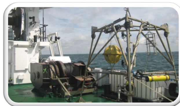
FIGURE 1. Benthic bottom lander, used in the Belgian nearshore area.
