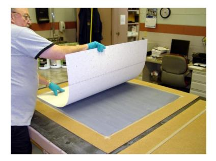
Figure II. Test Floor Preparation - #165 Adhesive
