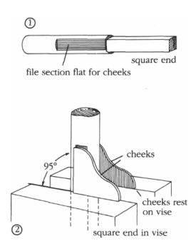
FIGURE 36. Preparing the mast for cheek installation.
