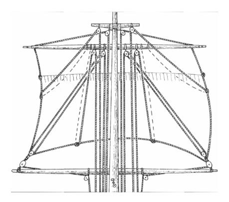
FIGURE 59. Yards were given a multitude of fittings to accommodate the spider's web of rigging needed to raise or lower sails. Why display full sails on your model after all the work of rigging the yards?
