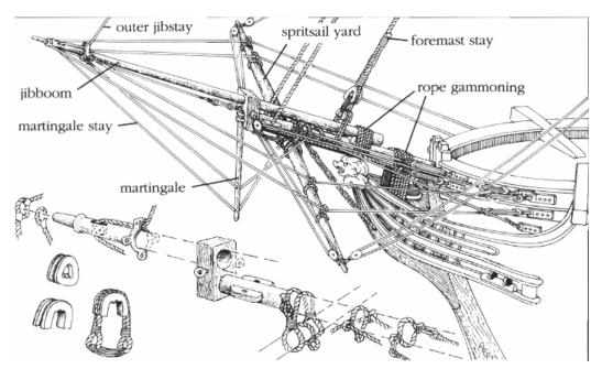
FIGURE 33. Bowsprit rigging evolved as structural strength and more efficient use of the wind became increasingly important. Earlier bowsprits relied on rope fastenings; later bowsprits used metal fittings and chain rigging.
