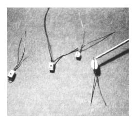
PHOTO 24. Blocks rigged with wire. Notice the tip of the awl inserted in the block's becket.
