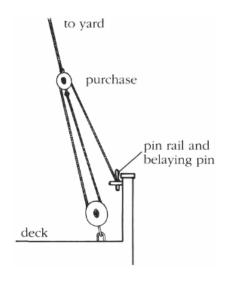
FIGURE 46. Halyards run through blocks on deck; a blessing for seamen raising and lowering sails.
