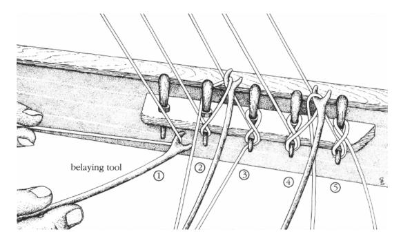
FIGURE 64. Belaying lines to pins—make yourself a belaying tool and follow this sequence from left to right.
