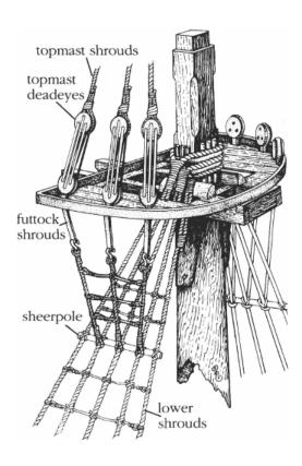
FIGURE 48. Futtock shrouds, iron rods or rope shrouds through the masttopplatform, countered the pull of the upper shrouds, adding stability and balance to the mast.
