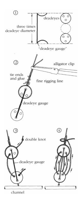
FIGURE 63. Rigging shrouds the easy way.
