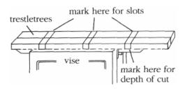
FIGURE 38. Precision cutting is vital when aligning crosstrees and trestletrees; a vise helps.
