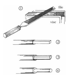
FIGURE 34. Reducing the lower end of the mast
