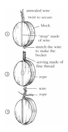
FIGURE 47. Securing blocks.
