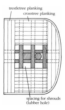
FIGURE 39. Planking the masttop.
