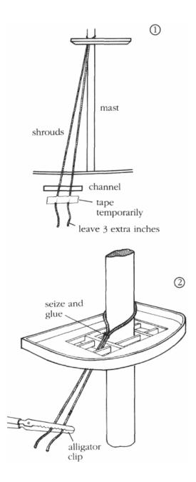
FIGURE 50. Rigging lower shrouds.
