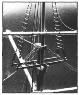
PHOTO 23. The masttop of a schooner. Notice the small rings below the deadeyes at the ends of the crosstrees. The futtock shrouds will be tied to these rings after the main shrouds are rigged.
