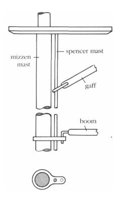
FIGURE 44. The smaller spencer mast made it easier to attach gaffs.
