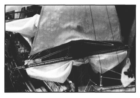
PHOTO 25. Sails are rigged to the yards with a running stitch — a relatively simple operation. Notice how a furled sail can help you show off your rigging.
