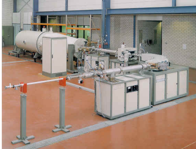
Fig 3 One possibility for a heavy-ion accelerator is a single-ended Dynamitron similar to that shown here.
