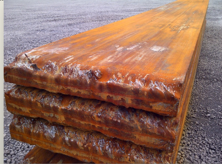
Slabs scarfed on a typical “Letter Box” Scarfer
