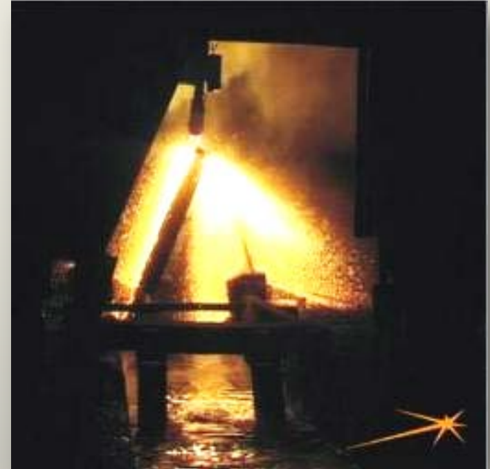
Slab scarfing showing the near vertical slab on the transfer car
