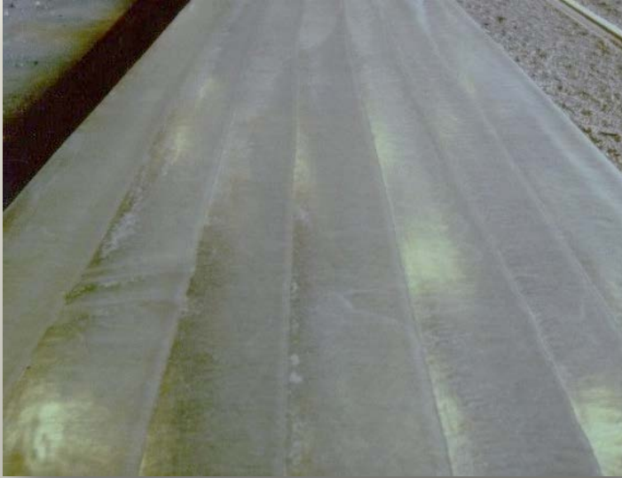
Slabs scarfed on the Evertz Scarfing Machine
