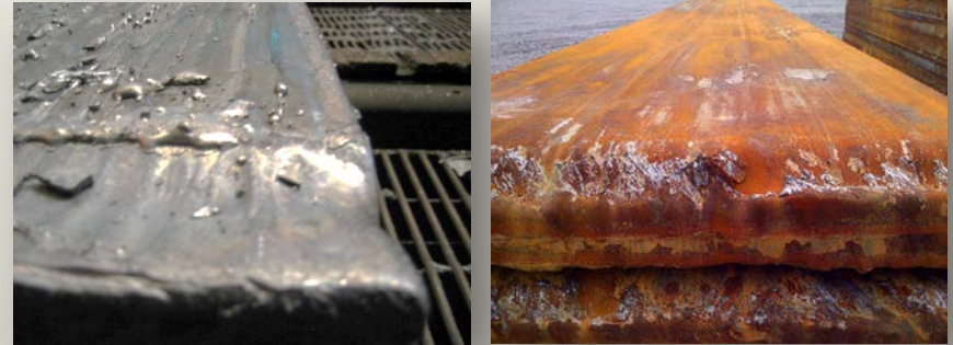
Slabs scarfed on a typical "Letter Box" Scarfer
