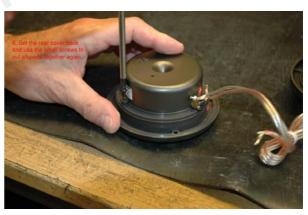
6. Reinstall the rear chamber and use the screws to put all parts together again.
