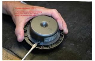
1. Remove the rear chamber by bending with a screwdriver on the three spots where it is attached to the driver. Be careful!
