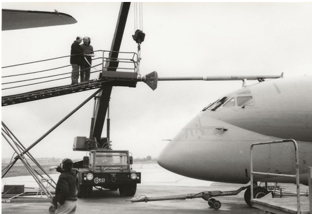
Positioning the Victor's refueling basket onto the Nimrod's probe
