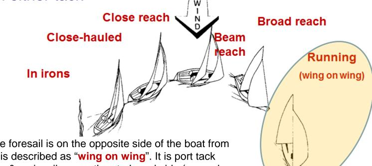
In this diagram the foresail is on the opposite side of the boat from the mainsail so it is described as "**wing on wing**". It is port tack because the boom & mainsail are on the starboard side (secondary definition of which tack the vessel is on)
