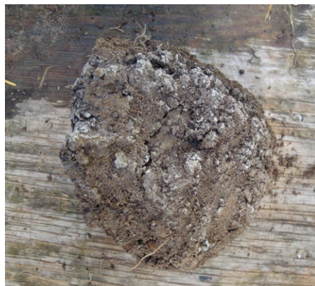
A sample of the saltpetre earth showing white crystals on the surface
