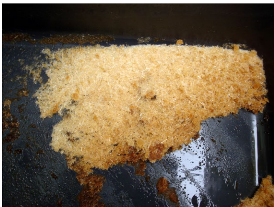
The needle-like crystals of saltpetre
