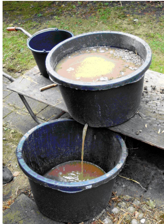
The tub was left for a period of time before the plug was removed and the water with the dissolved salts was allowed to drain into a bucket.
