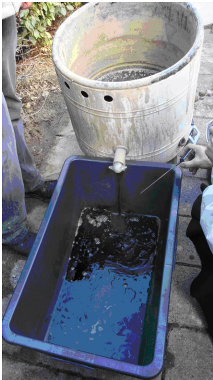
The final boiled down liquid being run into a tray for precipitation
