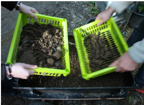
Sieving the raw saltpetre earth to break it down into smaller pieces
