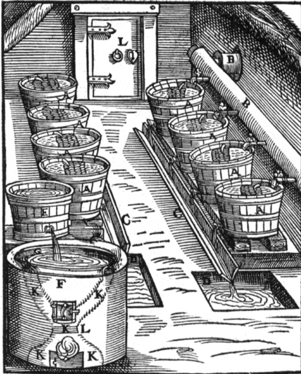
The method extracting and boiling down. From Ercker
